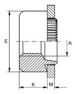
Female thread A = M2 Height K = 2.0 Outer diameter E = 5.0 Plate thickness = 0.7 Recommended bore diameter +0.05 = 4.0
